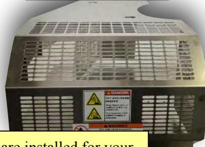
Feed Tray Guard and Mold Plate Guard are installed for your safety. Do not tamper with them in any way!
