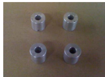
(4) Spacer Stanchions. Used for different Mold Plate thicknesses. May Be Plastic
